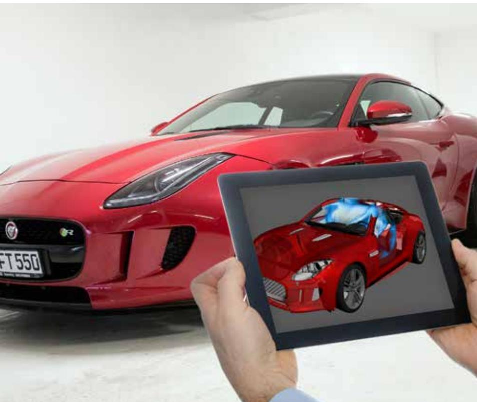
At Jaguar Land Rover, STAR-CCM+ is central in the design process of all current and future vehicle programs. Shown here is a cabin comfort analysis of an F-type luxury vehicle from JLR.
