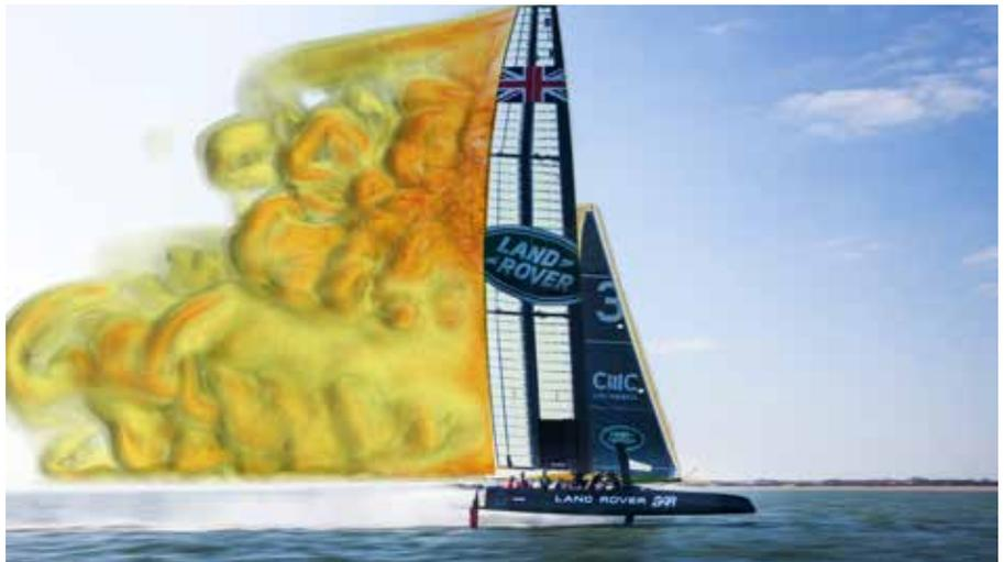
Design exploration with STAR-CCM+ has helped Land Rover BAR find the best possible compromise between aerodynamics and hydrodynamics for the America’s Cup racing yacht.
